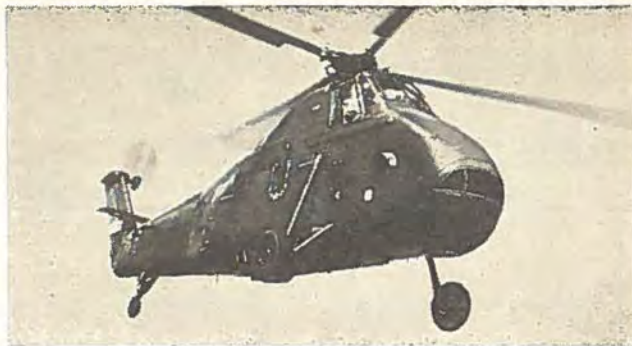
The Westland Wessex Mk.2, powered by coupled Gnome engines, under development for the Royal Air Force.
