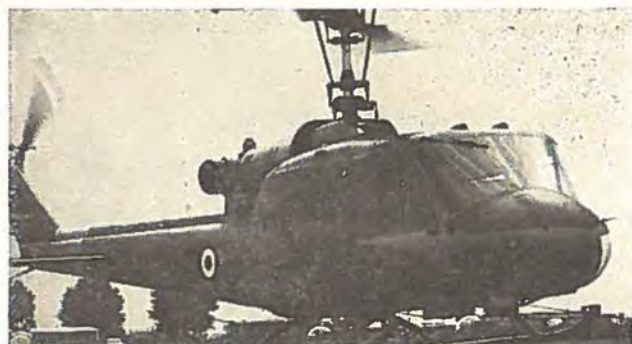
One of the Gnome-powered Agusta Bell 204 B helicopters for the Italian Air Force.
