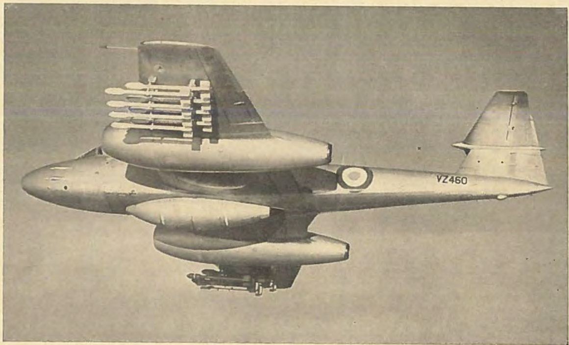
THE GLOSTER METEOR 8, TACTICAL GROUND ATTACK FIGHTER powered by two Rolls-Royce „Derwent“ turbo-jet engines
