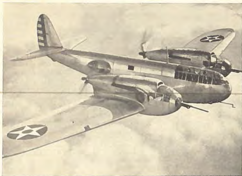
BELL XFM-1 tomotoret, tung Jager, hvis Motorer driver to Trykpropeller.
